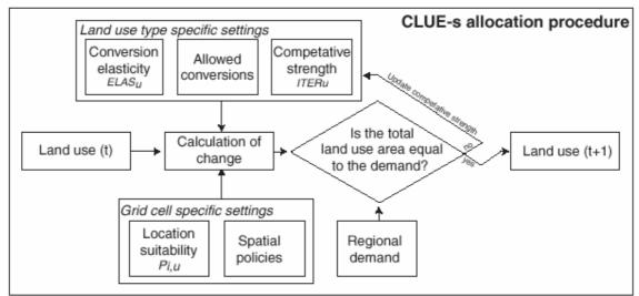
Figure 4.12 Flow chart of the allocation module of the CLUE-S model.
