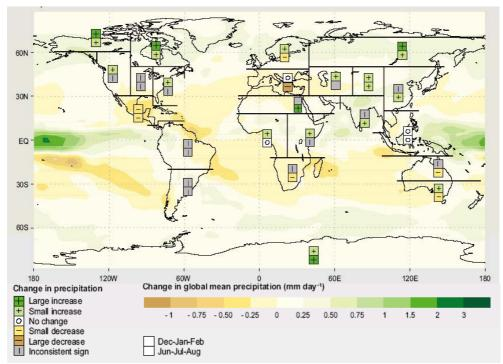
Figure 6.8b: Precipitation change for the 2080s relative to the averaged period between 1961 and 1990 for a high emission scenario (A1 or A2). Results are based on results from several General Circulation Models.
